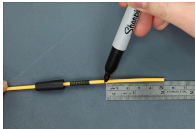
Step 2: Mark cable at 5cm.
